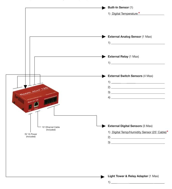
**Note:** The total sensor capacity of the Room Alert 12S is 11+ sensors.
